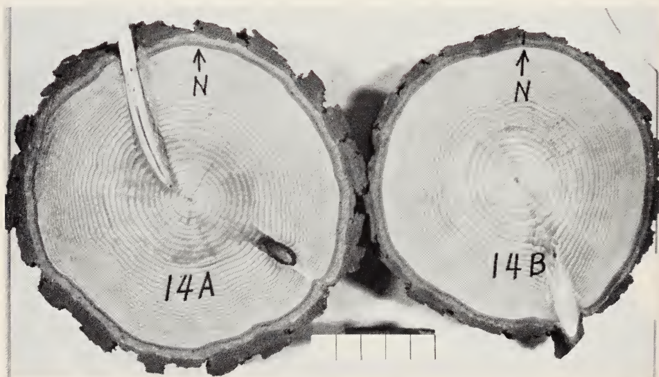
Fig. 2. Cross sections of young-growth tree 14 at large and small end of first 4-foot bolt.
